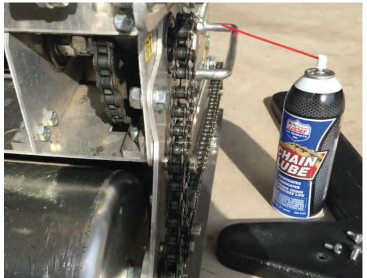
Lubricate three chains. Upper idler sprocket will adjust to tension roller chain.
