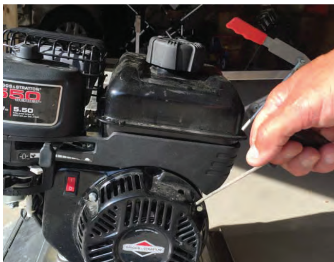
Turn off fuel, find top dead center of piston, place blocking on floor, and tilt machine for service.
