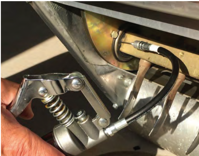
Grease four tine shaft bearings with a small grease needle
