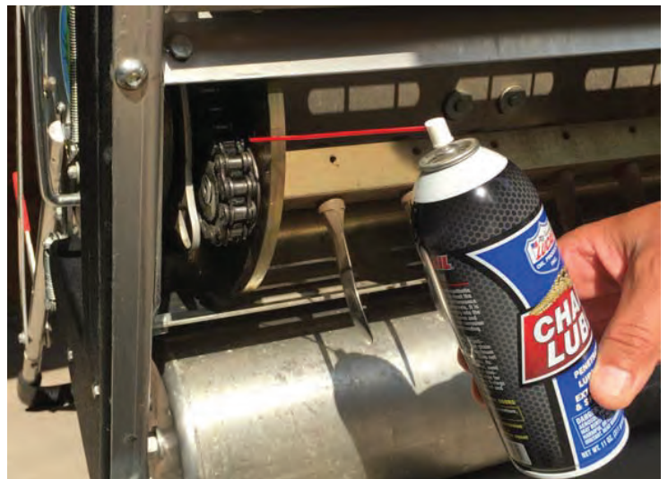
Lubricate three chains. Upper idler sprocket will adjust to tension roller chain.
